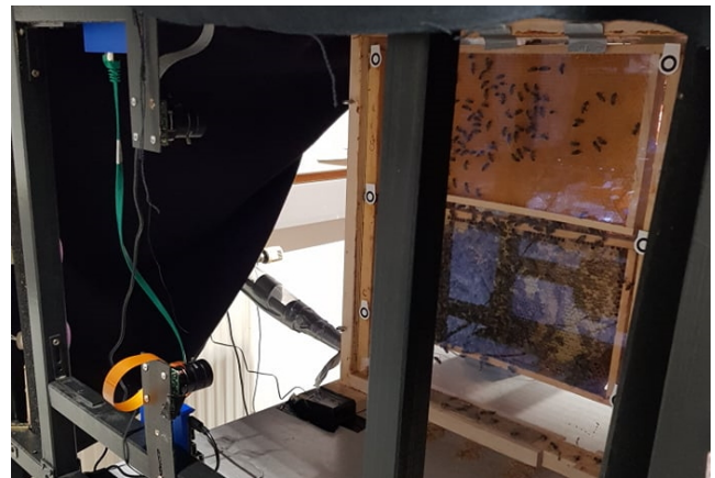
Fig. 2. Observation hive setup - two infrared cameras on the left are recording two combs on the right.
